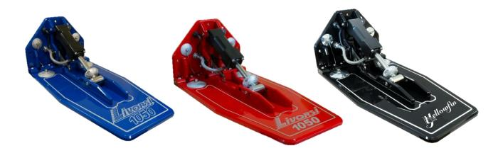
Livorsi's billet trim tabs stretch across the boating spectrum; models are available for performance boats, center consoles, cruisers, workboats, run-abouts and military boats from 20 to 50 feet and for use with 12 and 24 volt configurations.
